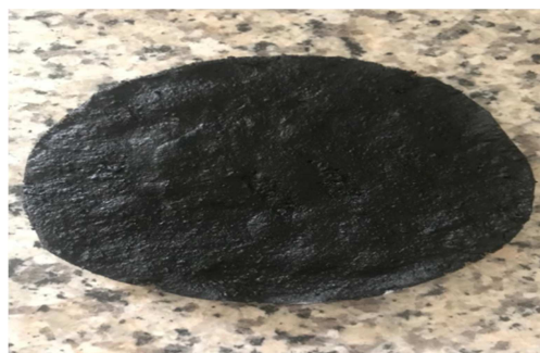
Figure 2. Banana Peels Bioplastic.
