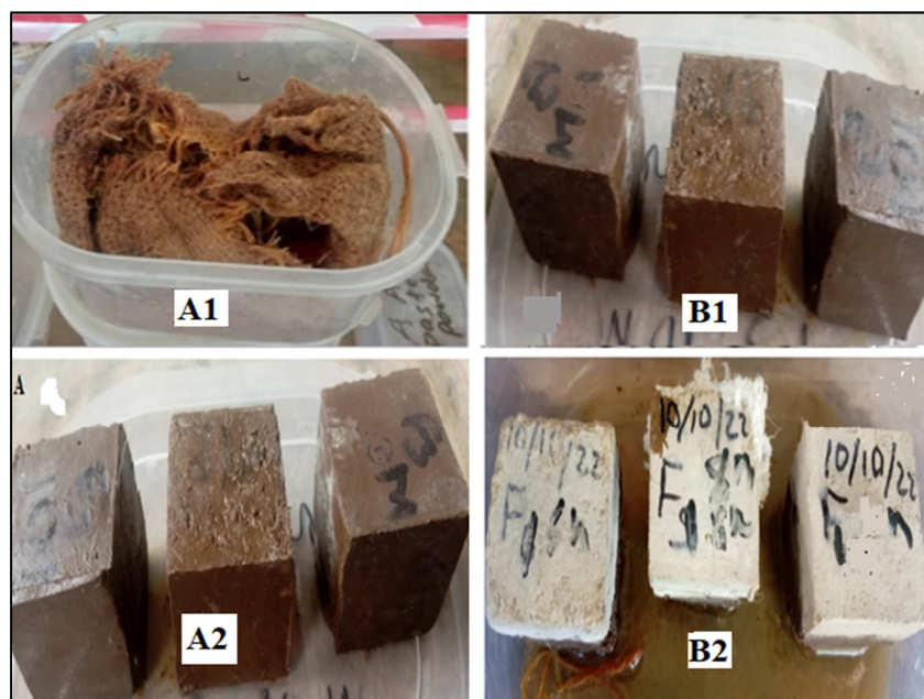
Figure 1. Photo A1 are specimens wrapped with wet hessian, A2 are 7 days specimens cured under wet hessian, B1 are quarterly immersed specimens in water and B2 are the 7 days half immersed specimens in water.
